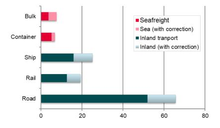
Figure 2-6 CO<sub>2</sub> emission factors 2015 (T2W) in g/tkm by transport mode (correction for partial load / empty return trips).
