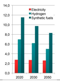
Figure 3-10 Production costs for electricity, hydrogen and synthetic fuels (in € ct/kWh) for different years, 8 000 full load hours, reference scenario (data from Agora 2018)
