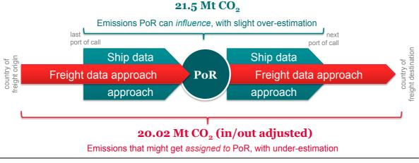
Figure 2-4 Two approaches for the assessment of CO<sub>2</sub> emissions of maritime transport in relation to the Port of Rotterdam
