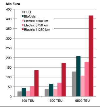
Figure 3-9 Energy costs for 20 years for different ship sizes and ranges (electric includes battery costs) (HFO 4.2 ct/kWh, Biofuels 7.0 ct/kWh, Electricity 4.0 ct/kWh)
