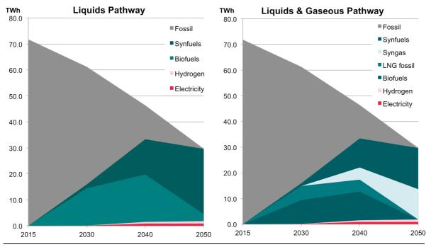
Figure 3-12 Amount of fuels used for maritime transport to and from Rotterdam 2015 to 2050 (TWh, T2W), two pathways
