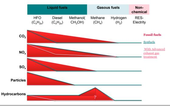
Figure 3-8 Emission characteristics of different fuel types
